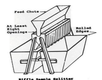
(a) Large Sample Splitter for Coarse Aggregate
